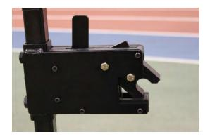
When the latch is open, the release lever is almost straight up and down. You must have the latch in this position when placing the racing chair on the roller.
