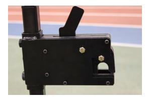
When the latch is closed, the release is angled towards the front of the roller. This is the LOCKED position that is required to be able to train safely.
