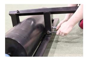
Insert the T-post into the back of the three post frame. Use your allen key to tighten the set screw into place. This will need to be adjusted once you place your chair on the roller.
