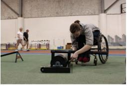
Place the front V-shaped frame under the end of the three post frame. There are different holes to line up depending on how long your racing chair is. To determine its length, measure from the hub of your back wheel to the hub of you front wheel. Then take that measurement and measure from the centre of the roller to the end of the V-shaped front frame. You only need a little bit of extra frame at the front. Once you have lined up the correct holes, slide the black bolts
