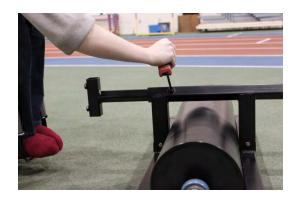
Insert the straight post through the T-post. Let the straight post come through showing 1-2" at the bottom. Use your allen key to tighten both set screws in place.
