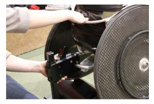
Loosen the set screw on the three post frame. Once loosened, pull the frame back, or push forward to align the hub of your back wheel with the bearing on the roller. You may need to tighten and loosen a few times before this is set up right, unless you have a helper that can watch the alignment while you use the allen key!
