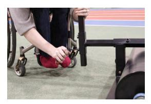
Place the latch on from the top of the straight post. Holding it 2-3" from the top, use your allen keys to tighten one or both set screws. Later, you will likely need to adjust the height of the latch to accommodate your chair.
