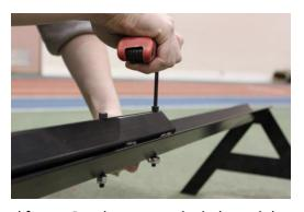
from the top of the three post frame through the V-shaped frame. Put the nuts on the bolts and then use your allen key and 7/16" wrench to tighten them.
